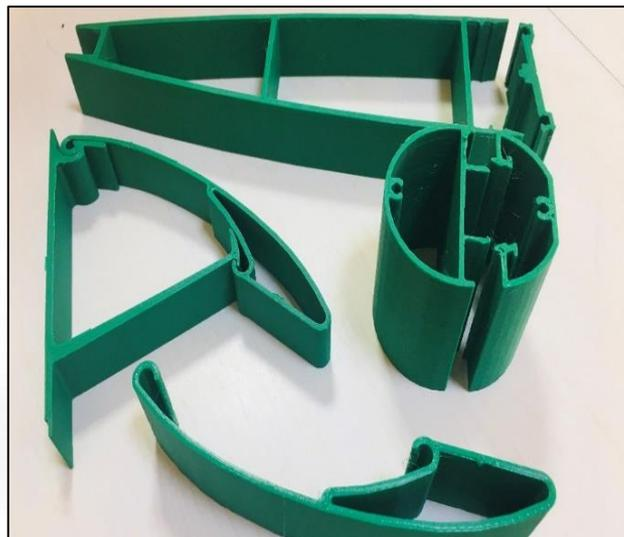
With our 3D-printing technology our customers can test the product for snap/slide fitment or gasket development prior to die manufacturing
